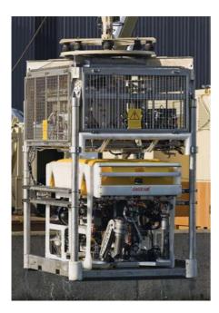
The TMS10 is fitted as standard with two camera and two LED light interfaces. Additional cameras and lights can optionally be added.
